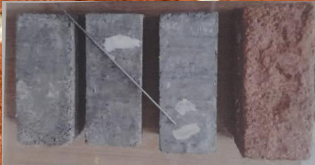
Waste plastic bricks with traditional brick
