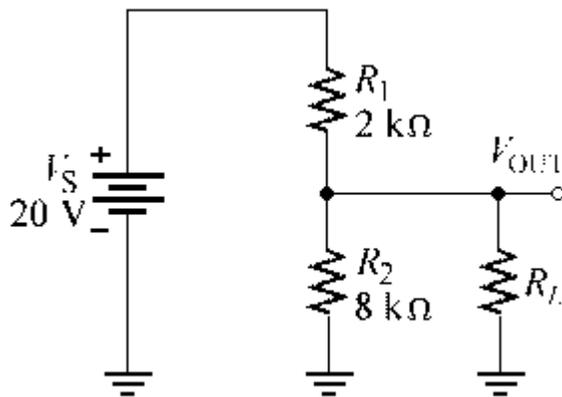
If the load in the given circuit is  $120\text{ k}\Omega$ , what is the loaded output voltage?
