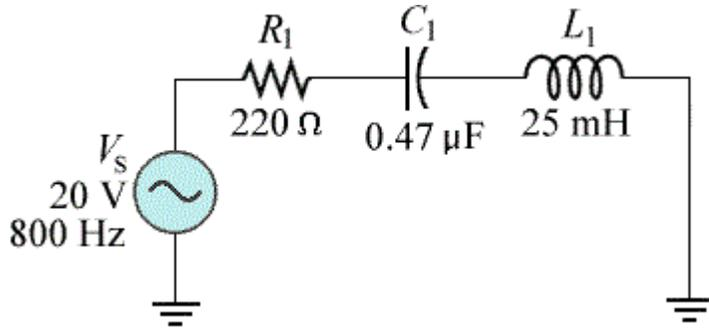
What is the impedance of the circuit in the given circuit?
