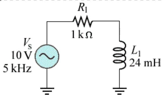
The voltage dropped across the resistor in the circuit in the given circuit is approximately equal to \_\_\_.
